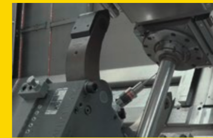
This is done with different B-axis angles and different clamping states (milling spindle clamped/unclamped, B-axis clamped/unclamped, ...).
