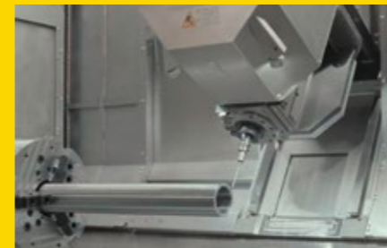
The X and Y axes are checked against the zero point. After inserting a short workpiece into the chuck, the headstock alignment is checked automatically.
