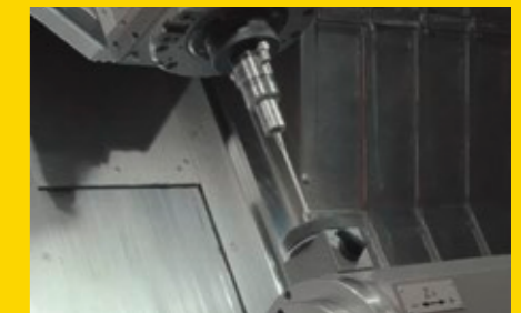
The repeat accuracy of the probe is then checked using the calibration ring. The workpiece probe is calibrated and checked for repeat accuracy.
