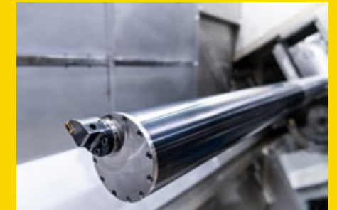
Standard tools can be used together with the prismatic tool interface with the WFL system boring bar.
