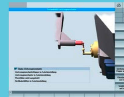
Turning, drilling and milling tools can be measured using the tool control cycles.
