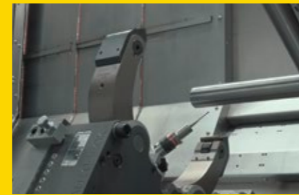
The concentricity and alignment of the milling spindle are measured with a test mandrel in the turning-boring-milling unit.
